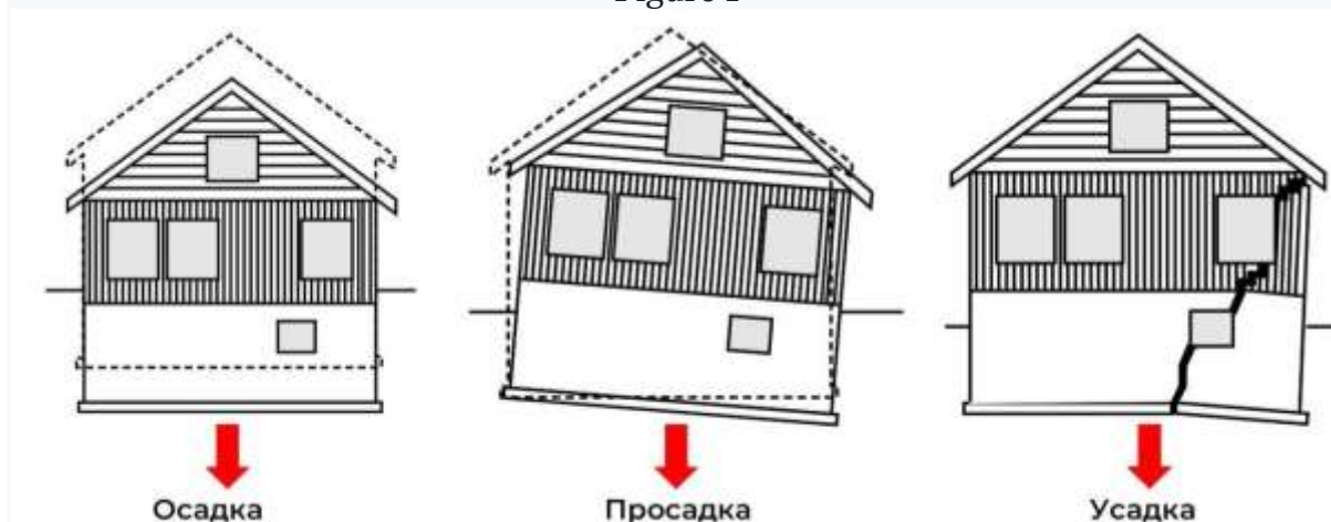
Figure 1. Sinking under load.
