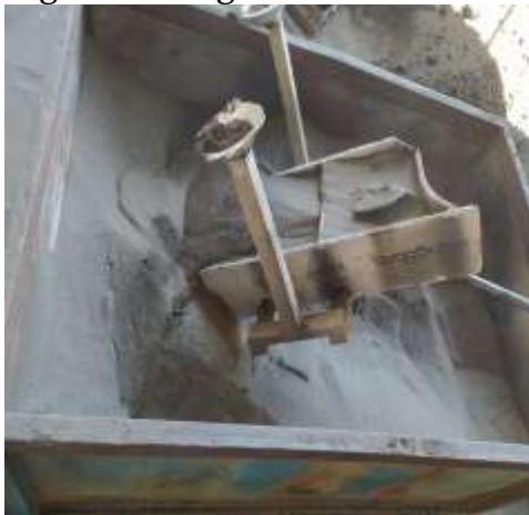
7 – picture. The process of extracting a casting from a mold with a special cell
