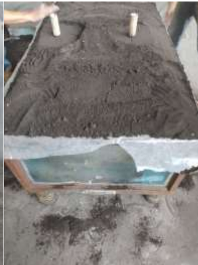
3 – picture. The process of placing the model in a mold with a special pocket 4 – picture. The ready state of the mold with a special pocket
