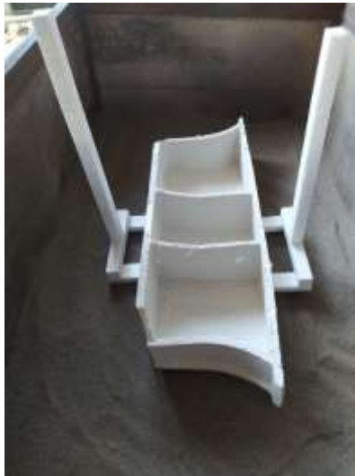
3 – picture. The process of placing the model in a mold with a special pocket 4 – picture. The ready state of the mold with a special pocket
