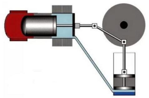
The piston mechanism provides for the use of two closed circuits: cold and with a displacer. Power is taken off a cold piston. The displacer piston is hot on one side and cold on the other. The heat exchanger is located both inside and outside the structure.
