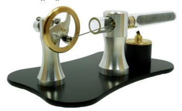
The engine uses acoustic resonance to carry out processes. The principle is based on the movement of matter between a hot and a cold cavity. The circuit reduces the number of moving parts, the difficulty in removing the received power and maintaining resonance. The design refers to the free-piston type of motor.
