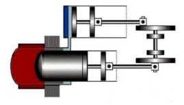
The design uses two different pistons placed in different contours. The first circuit is used for heating, the second circuit is used for cooling. Accordingly, each piston has its own regenerator (hot and cold). The device has a good power to volume ratio. The disadvantage is that the temperature of the hot regenerator creates design difficulties [6].
